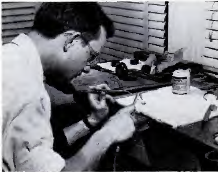
Second step in making ring is shaping silver band in circle and soldering at the joint with silver solder as shown here
